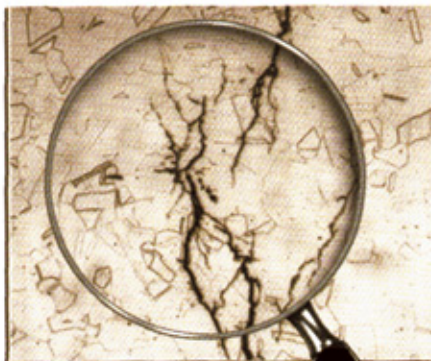
Microscopic cracking seen at 200x magnification.
